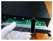
Fix the service board. Push the board down to the slot, and tighten the captive screws clockwise.
